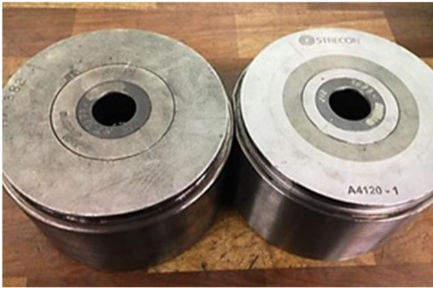
**Fig. 5** Cold extrusion tooling used in the experiments. Conventional shrink rings (left). STRECON system (right)
