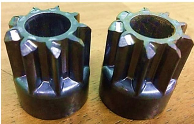
**Fig. 11** Pinions produced by cold extrusion with SAE 10B22 steel
